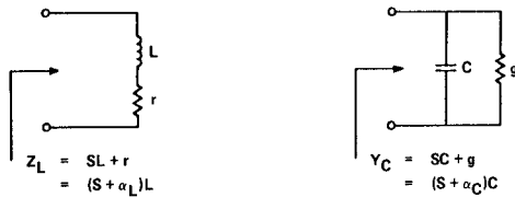
Fig. 2. Simplified equivalent circuit for lumped reactive elements.
